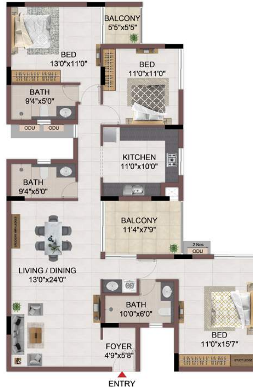
TYPICAL FLOOR 1ST TO 4TH
