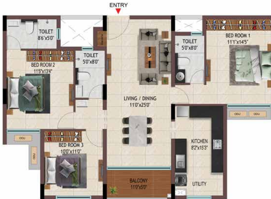
TYPICAL FLOOR (1ST TO 5TH)
